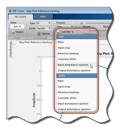
For example, to observe the closed-loop step response to disturbance at the plant input, in the **Step** section of the **Add Plot** menu, select Input disturbance rejection. The disturbance rejection response appears in a new figure.
