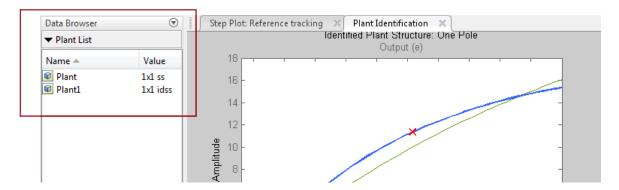
You can define the model structure and initialize the model parameter values using one of these plants. To do so, in the **Plant Identification** tab, in the **Structure** menu, select the linear plant model you want to use for structure an initialization.
