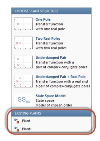
If the plant you select is a process model (idproc object), **PID Tuner** uses its structure. If the plant is any other model type, **PID Tuner** uses the state-space model structure.
