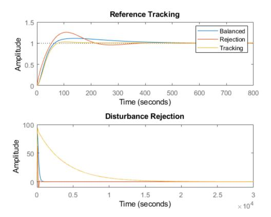
When you use the <code>DesignFocus</code> option to favor reference tracking or disturbance rejection in the tuned control system, you can still adjust phase margin for further fine tuning of the balance between these two measures of performance. Use <code>DesignFocus</code> and <code>PhaseMargin</code> together to achieve the performance balance that best meets your design requirements.
