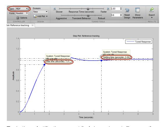
The rise time and settling time now meet the design requirements. You can use the **Response time** slider to make further adjustments to the response. To revert to the default automated tuning result, click **Reset Design**.
