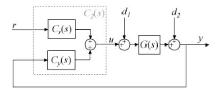
The system responses are based on the decomposition of the 2-DOF PID controller,  $C_2$ , into a setpoint component Cr and a feedback component Cy, as described in "Two-Degree-of-Freedom PID Controllers".
