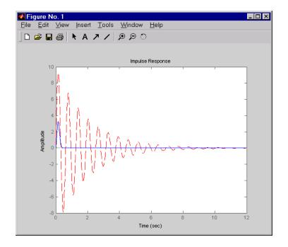
**Comparison of Open- and Closed-Loop Impulse Response**
