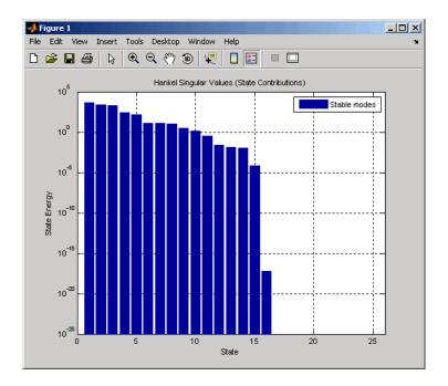
Small Hankel singular values indicate that the associated states contribute little to the I/O behavior. This plot shows that discarding the last 10 states (associated with the 10 smallest Hankel singular values) has little impact on the approximation error.
