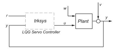
The plant has three states (x), two control inputs (u), two random inputs (w), one output (y), measurement noise for the output (v), and the following state and measurement equations:
