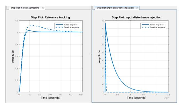
The PIDF controller tuned with reference-tracking focus is displayed as Tuned response (solid line). The plots show that the resulting controller tracks the reference input with considerably less overshoot and a faster settling time than the balanced controller design. However, the design yields much poorer disturbance rejection.
