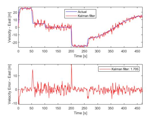
The legend on the error plot shows the east velocity estimation error  $||\dot{x}_e - \dot{\hat{x}}_e||_1$  normalized by the number of data points.
