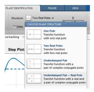
For any chosen structure you can optionally add a delay, a zero and/or an integrator element using the corresponding checkboxes. The model transfer function configured by these choices is displayed next to the **Structure** menu.
